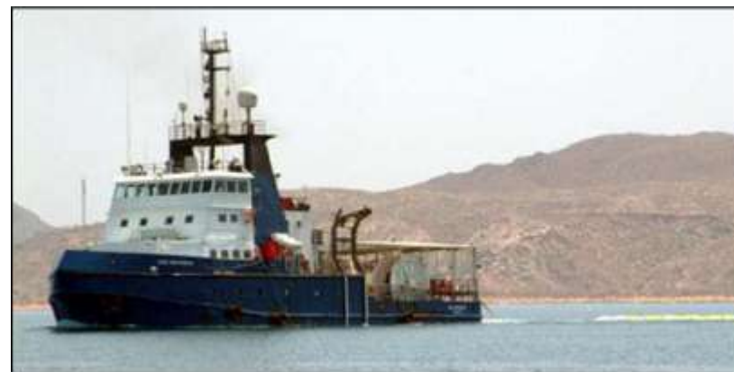
MV Geomariner – a shallow draft 2D/3D seismic vessel with a max draft of only 2.9m, able to operate in depths as shallow as 4m, used along coastal East Africa 2005 – 2007.
